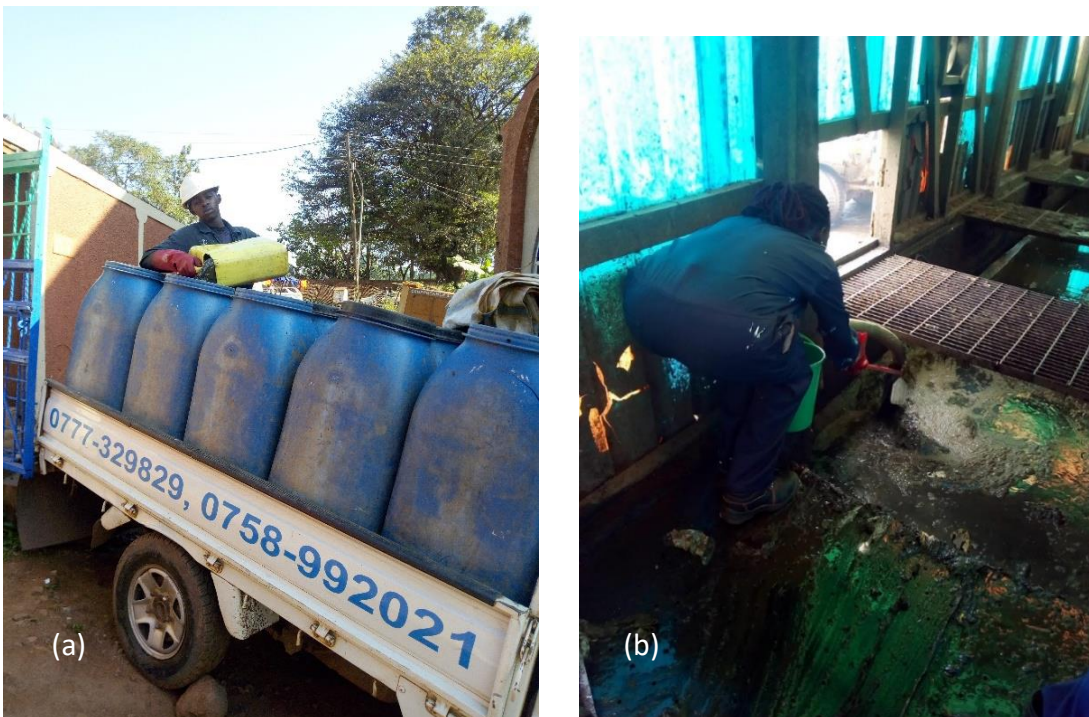
Appendix Figure E-2: Barrels of faecal sludge (a) and collection sample from cesspool truck (b)
