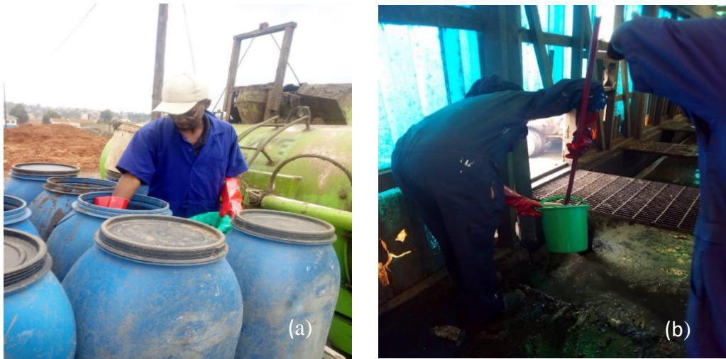
Figure 3-4: Sampling from barrels (a) and cesspool trucks during discharge at the treatment plant (b)
