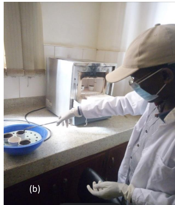
Appendix Figure E-4: Samples for laboratory analysis (a) and using muffle furnace for Total volatile solids analysis (b)
